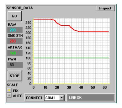
The laser power should be adjusted such that the receiver of the A-LAS sensor is not in saturation (A/D value >240).
