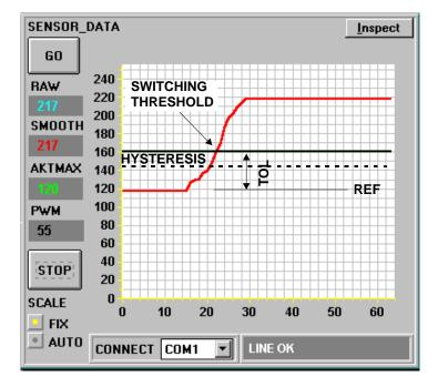
For example the target (reference part, accept part) is placed in the light measuring section of the A-LAS sensor in such a way that the covering by the target results in a raw signal value at the receiver of approx. 120 A/D units (light measuring section covered half). This value of covering is declared as the reference value, in this case e.g. REF=120.
