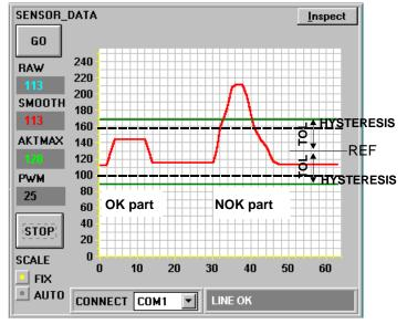
The target (reference object, accept part) is placed in the light measuring section in such a way that the light measuring section is covered half (reference value REF=128). The intensity detected at the receiver of the A-LAS sensor is proportional to the covering at the light measuring section.
